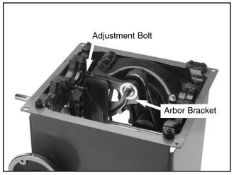
Figure 29. Adjusting arbor bracket.
